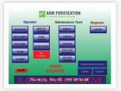
Main entry screen, with options for three levels of password protected operation.
